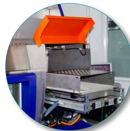
Two different sample racks are supplied: a) rack with 56 positions for 20 ml and 40 ml (new) sample bottles.
