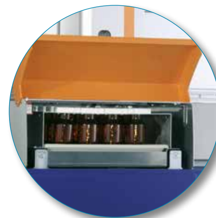
b) Rack with 16 positions for 100ml sample bottles and viscometer with standard sample volume and rinsing with sample
