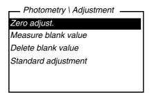
3 Using <▲> <▼> and <START/ENTER>, select and start the *Zero adjust.* function.
