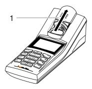
Inserting a 28 mm cell
