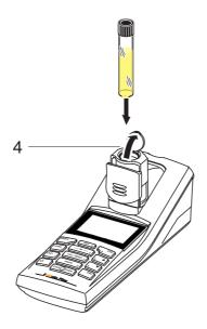
4 Insert the 16 mm cell (marking points to the front) so that it is positioned on the bottom of the cell shaft.
