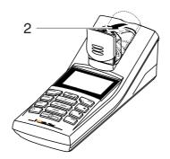
2 Pull upwards the height adapter (3). The cell shaft is extended.
