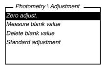
4 Using <▲> <▼> and <START/ENTER>, select and start the *Measure blank value* function.
