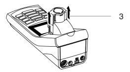
Open the external light cover (4) of the cell shaft.
